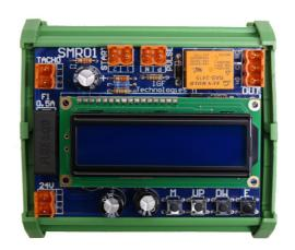
The Speed Monitoring Relay SMR-01 is specially designed for escalator applications. The range of the voltages and frequencies for monitoring are broader than the escalator ones and this unit can be used in variety of other applications. All parameters can be easily set via four push buttons and LCD display.
